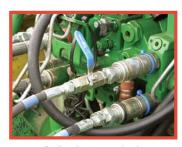
Ball valve wing lock up system
