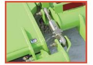
Greasable adjustable turn buckles for parallel levelling
