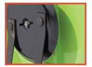
7 gauge spun formed stump jumper pans
