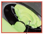
Metal seal guards on 517 hubs
