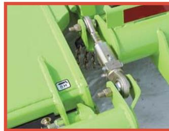
Greaseable adjustable turnbuckles for parallel levelling
