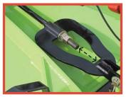
Single levelling rod with floating hitch
