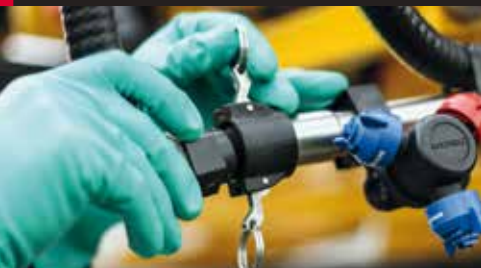
Spray line quick release drain point
