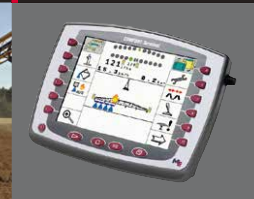
Automatic spray controller
